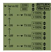
The direction of rotation of the servo can be reversed (servo reverse) by entering a negative value for the mix rate. Simply tap on the value (prefix reverse) to change the direction of servo rotation.
