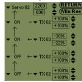
This function is used to distribute and assign the servo outputs to the functions controlled by the transmitter; this is a facility which offers important advantages when programmed at the receiver. For example, in this case transmitter channel 1 operates the servos at receiver outputs 2 and 3 simultaneously, requiring no Yleads or mixers. Servo travel and direction are variable.
