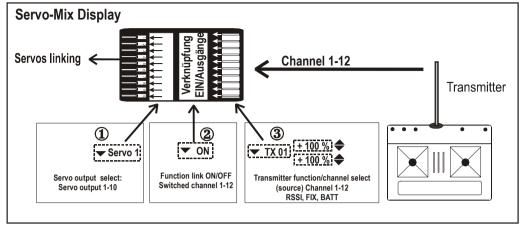
The DSL-system works in a similar fashion to any computer transmitter: **The servo outputs at the** receiver are linked to the transmitter's sticks / controls.
