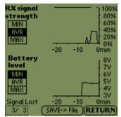
A very important function of the receiver is to record the reception conditions and battery status during the last 20 minutes of every flight. When the model is back on the ground, you can easily examine the receiving situation and battery voltage which occurred during the flight. The receiver stores a value for reception field strength every 20 seconds, and battery voltage every 60 seconds.
