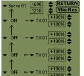
These settings (+ sub-trim, see below) are designed for matching servo travels, e.g. when one control surface is actuated by multiple servos. This function eliminates the problem of servos working against each other, causing them to draw excessive currents.
