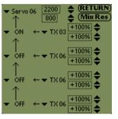
**Airbrake --> elevator compensation**, elevator is transmitter channel 2 and receiver output 2. Airbrake is transmitter channel 3 and receiver output 3. When you operate the airbrake channel, a compensatory elevator movement is automatically mixed in; the degree of compensation is set in the second line of the mixer.
