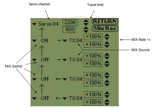
Every Servo-MIX display always refers to the servo (or corresponding receiver output) indicated for that servo channel (see diagram). Four mixers and two end-points can be programmed for all 10 servos which can be connected to the receiver. Each additional mixer function is added to the first mixer function.
