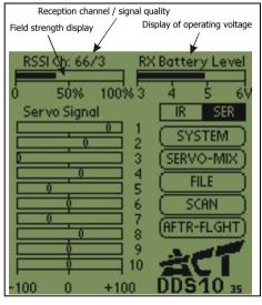
The buttons SER (serial) and IR (Infra-Red) are available for you to select the method of connection. If the receiver(s) is (are) connected via the Infra-Red Interface, you must also select the receiver connected in this way. You can do
