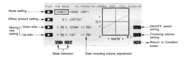
Use the A ( ) key to activate mode setting, then press the ACT or INH keys (F and G) to activate or inhibit flap-to-elevator coupling.
