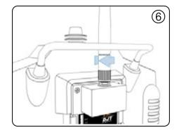
5 - Turn the transmitter on and check the LED status on the module. Normal operation on the transmitter is indicated with the RED LED on and the GREEN LED flashing.
