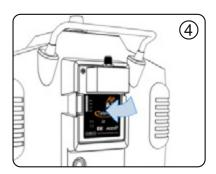
4 - Screw thoroughly the module antenna without undue stress:
