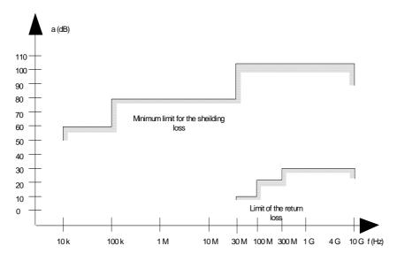
Figure B.2: Specification for shielding and reflections
