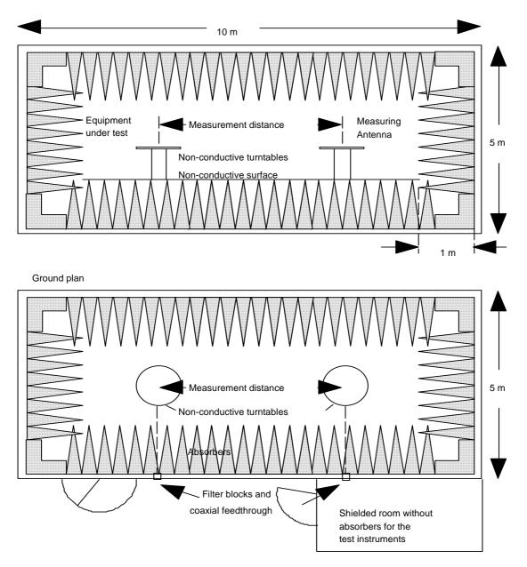
Figure B.3: Anechoic shielded chamber for simulated free space measurements
