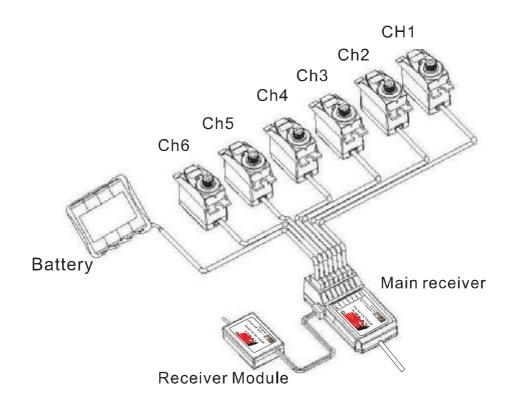
When installing the receiver please make sure that two items showed 90 degree angle.
