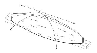
Gently apply resin or epoxy to the hull, starting in center of keel and work toward bow and stern. Apply resin or epoxy to the remainder of the hull using a downward motion and let cure. Note:
