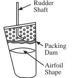
slightly below the rudder shaft. Align the shaft in the rudder so that it is at right angles to the water line of the hull, vertically straight with the rudder sides, also with about 60 % of the rudder area aft of the shaft. When it's in alignment tack glue it with Zap. Now you can fill the inside of the rudder with a filler of micro-balloons and resin or epoxy.
