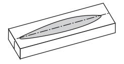
(this will very with bulb size) balsa wood together. A layer of thin cardboard lightly glued between the blocks makes splitting them apart much easier. The glue joint will be broken apart later.
