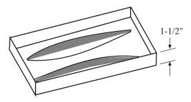
can speed up the process by using your kitchen oven. Three or four hours at 200 degrees F, maybe longer, should do the trick. Let plaster cool. Place plastic wrap (Saran, etc.) over plaster mold. This acts as a parting agent and allows the slugs to be removed from the mold easily.
