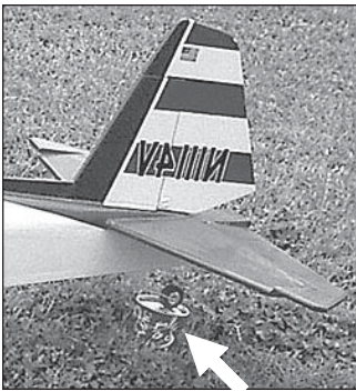
Prop tail of taildragger so fuselage is level
