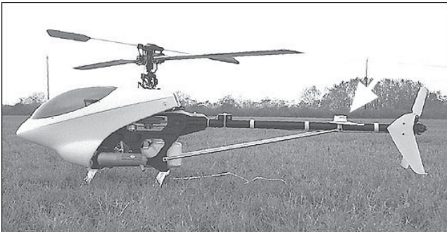
Helicopter level on grass. A bubble level (arrow) will enable you to position the helicopter accurately
