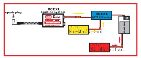
This device allows you to safely and remotely kill your electronic ignition equipped engine from your transmitter. This kill switch is Fiber Optically Coupled to isolate your ignition system from your radio system. (No Interference!!) this device features the following:
