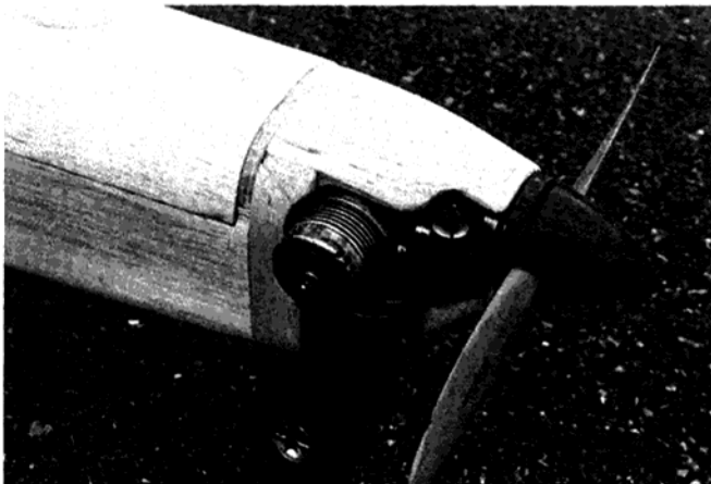
TOP LEFT: Major components. L.E. of stab tapered in final version. TOP RIGHT: Completed framed-up Headmaster Sport 40 ready for covering. CENTER LEFT: Tank and hatch detail. CENTER RIGHT: Hatch detail. LEFT: Side mounted engine is cowled in with balsa blocks.
