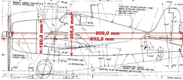
The overall length of the model is allowed to deviate by no more than 5%.
