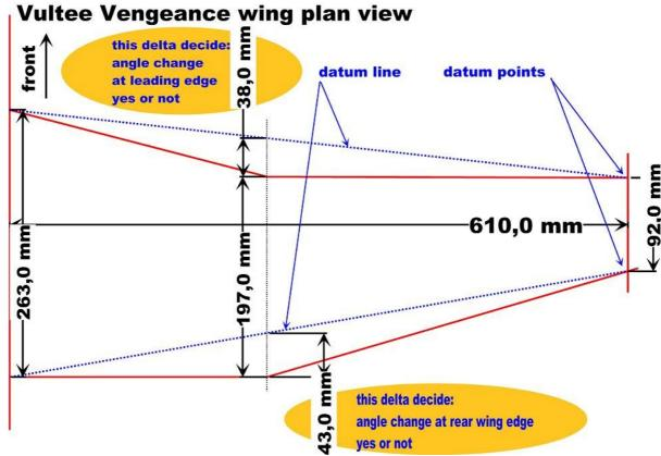
You can see clearly that there is more than 20mm deviation from the datum lines (----) at both the leading and trailing edges of the wing. This means your model should also be built with similar angle change.
