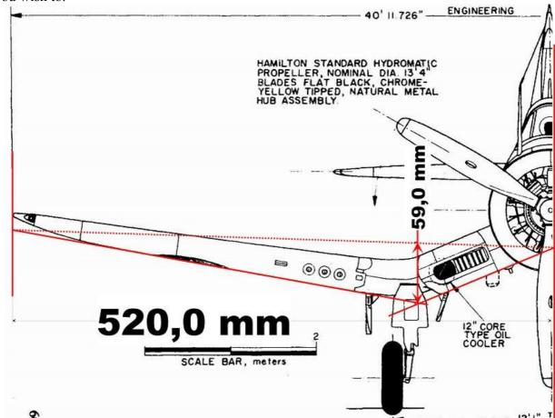
If we look at the drawing of an F4U Corsair, you can see the difference between the datum line (-----) and the bottom surface of the wing is more than the allowed 20mm deviation. In this instance you can see your model wing will need to be built with a crank/angle change to remain within the 20mm permitted tolerance.
