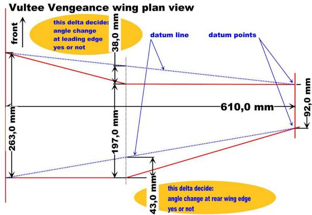
You can see clearly that there is more than 20mm deviation from the datum lines (----) at both the leading and trailing edges of the wing. This means your model should also be built with this angle change.
