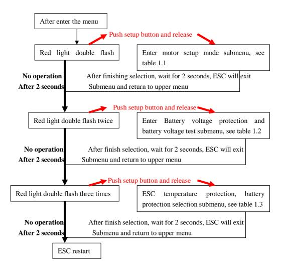
How to choose the right settings for you: When you enter each sub-menu, you can read current parameters by the different light combinations, for detailed information please see each data table. Within 2 seconds, you can change parameters by pressing the setup button, based on the light combinations in each data table. If there is no operation after 2 seconds, then the ESC will save current data and exit to next main menu. (Same process for all setups)
