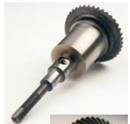
Above: here you can clearly see the rotating-sleeve/propshaft component. Note the single port cut into the large forward portion.
