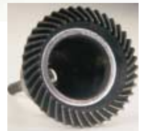
It acts as both the intake and exhaust ports. Left: at the aft end of the sleeve is a large helical gear. It mates with the small gear that's driven by the crankshaft at the back of the engine case.
