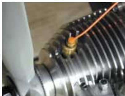
For safety, use a glow-plug extension wire and a remotely located glow-driver connector. The glow plug is extremely close to the prop, and you should not attach your Ni-Cd driver battery directly to the plug.
