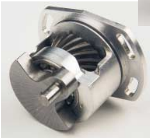
This assembly houses the crankshaft and crank gear as well as the support bearing and starting socket. The unit seats into the crankcase.
