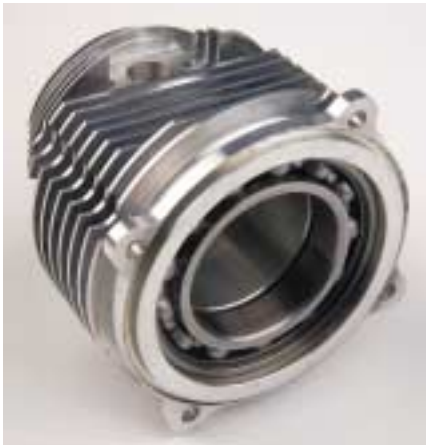
Above: shown here is the cylinder jacket or main engine case. Note the large main bearing that supports the sleeve and allows it to revolve. Below: the crankcase is CNC-machined from a large block of aluminum. It also serves as the engine's mount.
