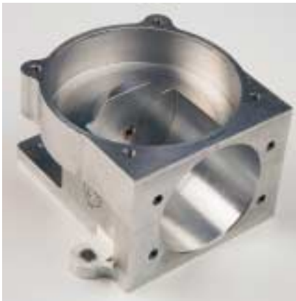
Above: shown here is the cylinder jacket or main engine case. Note the large main bearing that supports the sleeve and allows it to revolve. Below: the crankcase is CNC-machined from a large block of aluminum. It also serves as the engine's mount.
