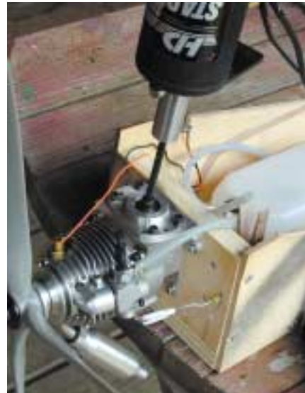
Only start the engine with the behind-the-prop-starting wand. It is both easier and safer to start the engine this way.
