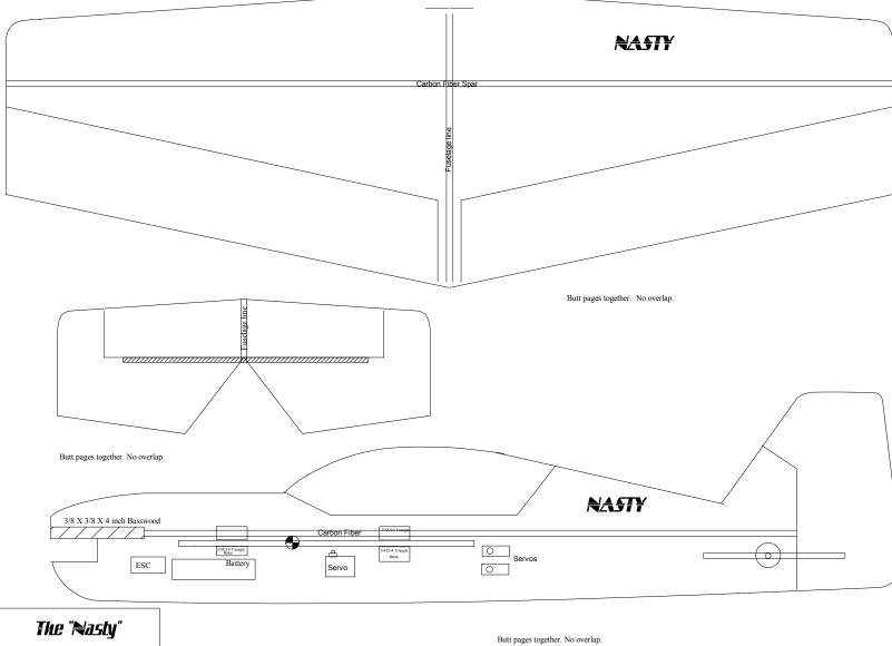
Wingspan- 38 in. Length- 36.5 in Weight- w/o batt. 10 oz. Motor- GWS350D/Razor 400 Prop- 11-12 inch Battery- 3 cell-850-1500 ma. Designed by Charles Pirkey Capyright2005
