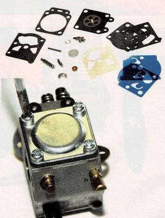
**STEP 6** In most cases, a good cleaning of the inlet side and possibly the replacement of the gaskets are all that's required to restore proper engine operation. If, however, that doesn't help, you can check the fuel-metering section by removing the other side cover that's held in place by four corner screws. Again, check for any obvious debris and give it a light spray of WD-40.
