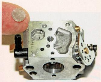
**STEP 5** Should you find that the filter screen is blocked with gunk or has trapped some dirt, clean it out with a quick spray of WD-40. If that doesn't do the trick, a replacement screen is included in most Walbro rebuild kits; these kits are available from gas-engine manufacturers as well as local small-engine shops. Some hot-shot pilots may suggest that you can discard the filter screen altogether, then use clean filtered fuel. I don't recommend this as the increase in fuel flow is minimal.
