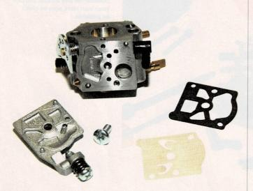
**STEP 4** On the inlet side of the carburetor body, removing the single center screw gives you access to the fuel-pump diaphragm, the gasket, and the unit's fuel-filter screen. Remove the screw and side cover, then inspect the thin diaphragm and the flapper tabs to make sure there is no deterioration. Clean out any obvious debris using the BBQ skewer. Don't use a sharp tool or a hobby knife as these can damage the surface of the passages.
