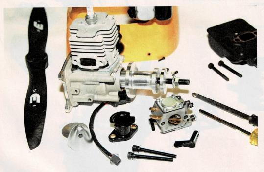
STEP 2 Here's the engine removed from the Piper Cub. I prefer to do this job away from the model to give me plenty of elbow room. Place the engine on top of a paper plate or a disposable foil tray so that you can keep your work area as clean as possible.
