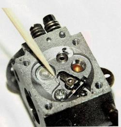
STEP 8 To avoid damage to the carburetor components, it's important to clean using only soft, nonmetal tools. Gasket scrapers, razor blades and any other sharp utensil can seriously harm the relatively soft aluminum that comprise the carburetor body and cover plates. Using them can lead to air leaks, which are not a good thing.
