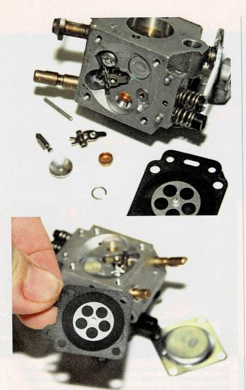
**STEP 7** Held in place with a small screw, the inner metering needle, spring, and lever arm can wear over an extended period. These parts automatically adjust the fuel flow to maintain proper fuel flow relative to outside atmospheric pressure. If these parts show wear, carefully replace them with the rebuild-kit parts. Use care, and don't force anything in place.
