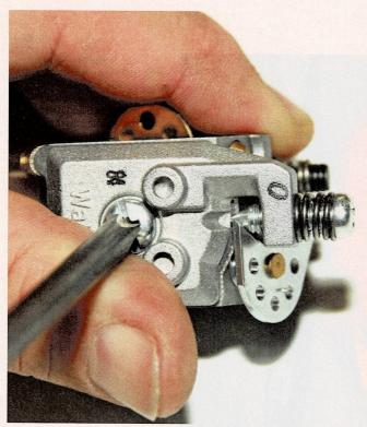
**STEP 3** Remove the carburetor from the engine. To do this, simply remove the two attachment bolts and the spacers from either side of the intake. Be careful not to damage the gasket. Unless your carburetor has suffered a major, muddy ground strike or encountered a severe fuel blockage, all you'll need to do is give the carburetor a good cleaning and possibly rinse out the main-filter screen.
