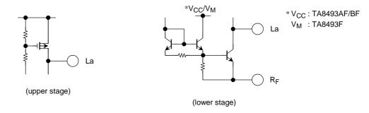
This circuit uses the system to chop the lower power transistors and resurrect coil current through upper stage diodes.
