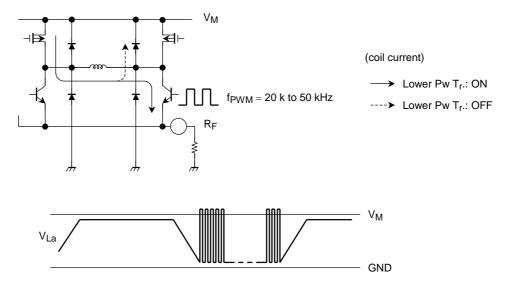
Note: Lower-stage predrivers of TA8493AF/BF are supplied by V<sub>CC</sub> to reduce the power dissipation.
