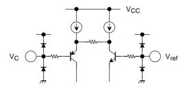
The common mode input voltage ranges for both VC and  $V_{ref}$  are 0.5 to 4.0 V. Relation between control input and PWM ON duty is shown below, PWM ON duty is 100% when  $|V_{ref} - V_C| = 0.75$  V (typ.)
