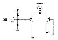
When the driver IC is standing by, all of its circuits except the FG amp and the hall amp are turned off.
