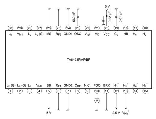
VHYS: Switch the VHb<sup>+</sup> from high (H) to low (L) and from (L) to (H). Measure the V<sub>Hb</sub><sup>+</sup> at the point when FGO function changes.
