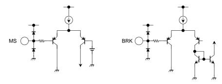
When  $V_C > V_{ref}$ , one of three modes (reverse rotation, reversing brake or short brake mode) can be selected by setting the MS and BRK pins appropriately.
