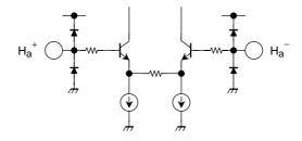
The common mode input voltage range for  $V_{\mbox{CMRH}}$  is 1.5 to 4.0 V.
