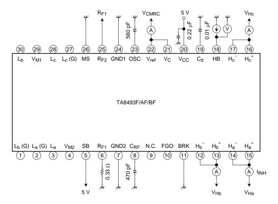
• IINH: Total of a phase negative and positive input current.
