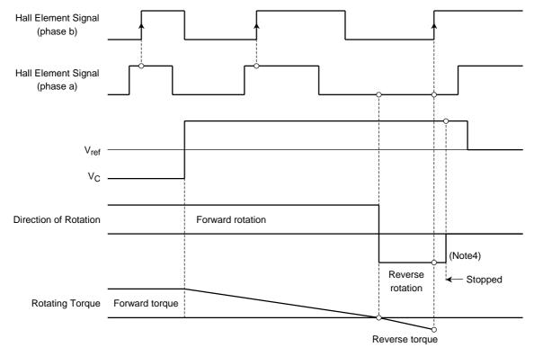
Note4: Due to its inertial force, the motor does not stop immediately after the torque is reduced to 0.
