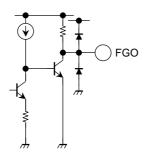
This circuit uses a hall element signal which is output to FGO after a Schmitt stage.
