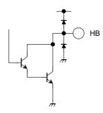
The hall element bias current is turned off when the driver IC is in standby state.
