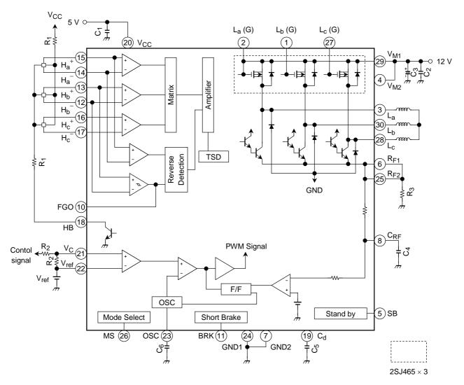
Note10: Utmost care is necessary in the design of the output line,  $V_{CC}$ ,  $V_{M}$  and GND line since IC may be destroyed due to short-circuit between outputs, air contamination fault, or fault by improper grounding.
