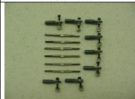
Aileron/Elevator Titanium rods & ball links
