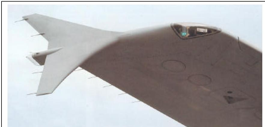
API claims that moving the winglet root forward also eliminates problems with small vortices that roll up from the highly swept wingtip area just ahead of the conventional winglet-towing junction at maximum chord thickness. Eliminating the roll-up vortex further reduces interference drag.
