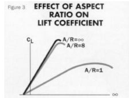
The desire for high aspect ratio and optimum aerodynamic efficiency must be balanced against other factors, such as material-strength-to-weight ratios, overall weight of the wing, internal fuel capacity and parasitic drag. For those reasons, the best aspect ratio for the average business aircraft wing might be seven or eight to one. For instance, the aspect ratios for the Hawker 800XP, Falcon 2000 and Beechjet 400A are 7.1, 7.6 and 7.8, respectively.
