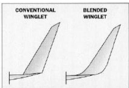
The comparison between the blended winglet and the conventional winglet shown in this illustration contrasts the large radius transition section and spanwise blending of the Gulfstream II winglet with the absence of a meaningful transition section for the conventional winglet. High aspect-ratio blended winglets have demonstrated they are 60 percent more effective than conventional winglets.
