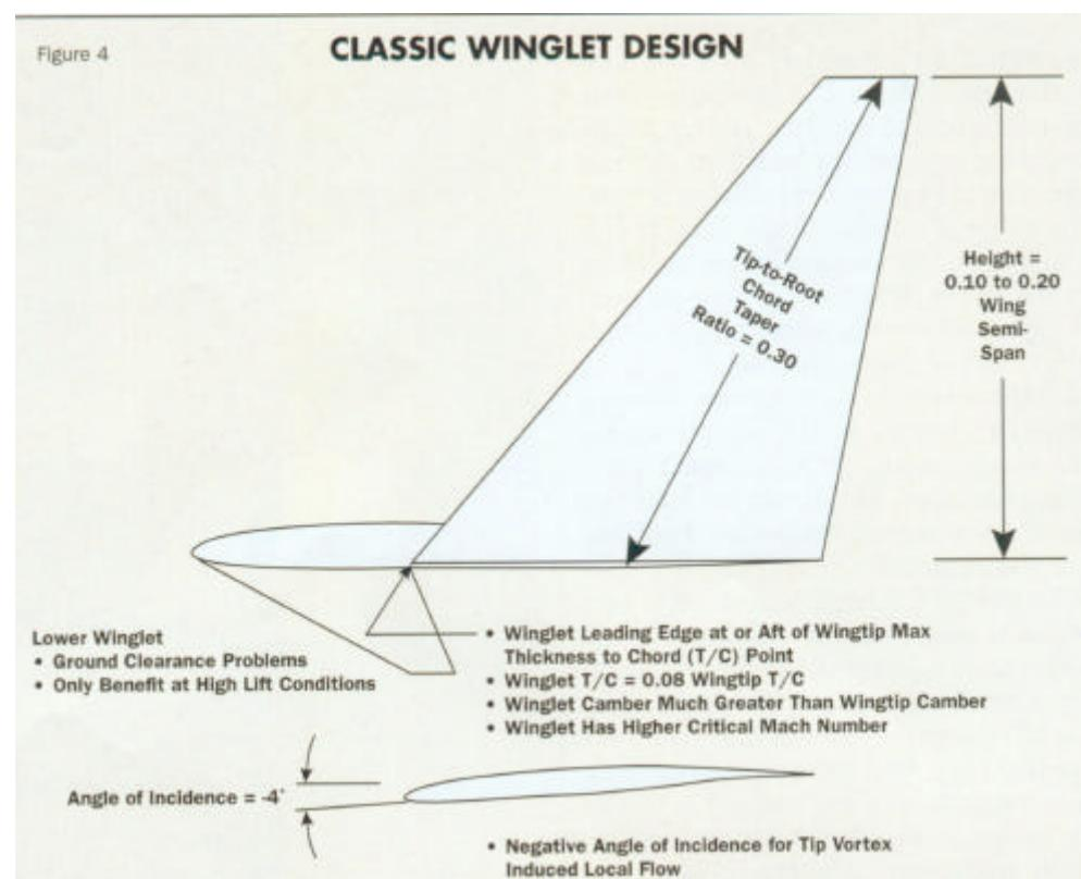
reduce it from reinforcing the shock wave of the main wing near the tip. Whitcomb chose an airfoil with significantly more camber than the wing, but with an eight percent thickness-to-chord ratio.
