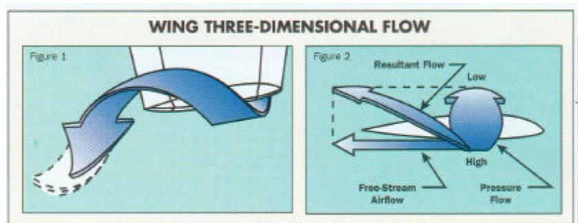
They induce a decrease in the angle of attack of the average relative wind flowing around the wing.
