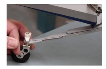
13. Use pliers to twist spring ends closed around the tillers after desired tension and direction adjustments are complete.
