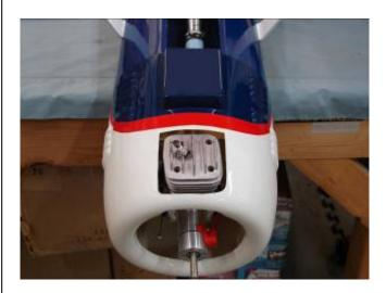
Cowl cut out for engine cylinder head with
