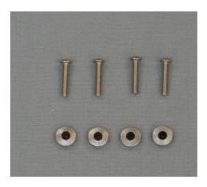
8. Slide the rubber backed washers on the hatch mounting bolts and insert bolts through the hatch mounting holes and into the fuse blind nuts. Tighten snugly but do not over tighten and crush the hatch or the fuse sides.
