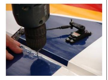
6. Mount the control horn using six wood screws as shown.
