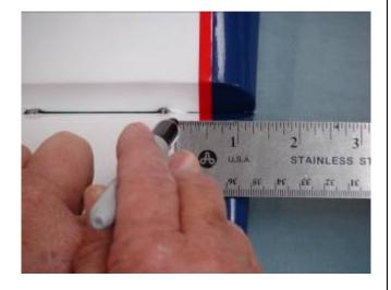
3. Center the rudder control horn over the mark and mark the locations of the control horn mounting holes.
