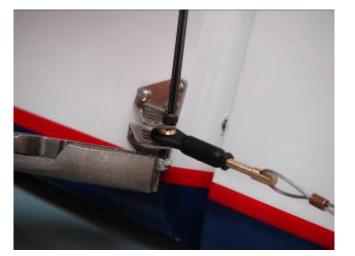
18. Adjust rudder pull-pull cables to desired tension by screwing in or out on the threaded couplers and or ball links. Make all adjustments with the rudder servos still powered up and centered, and the rudder still taped in the neutral position. Ensure the servo does not bind at center or at either end point.
