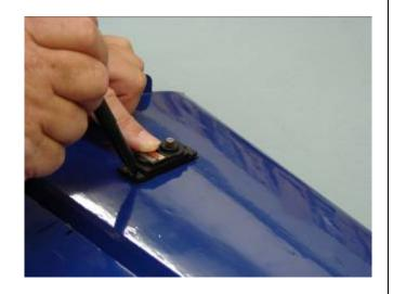
5. Remove servo and use a 1/16 bit to drill servo mounting holes.
