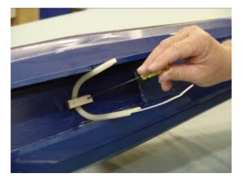
26. Allow the nylon tie lock to extend out of the tunnel 1/1/2" as shown. Tighten the mounting bolts securely.
