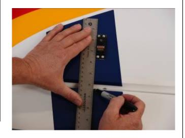
3. From that mark measure 1/2" toward the wing tip and mark the leading edge of the aileron as shown. This mark will be the center of the aileron control horn.
