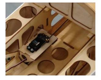
14. We recommend installing the carburetor choke pushrod as shown. Use nylon ties to provide support and holding friction for the choke pushrod. Place silicon fuel tubing over the wire pushrod to prevent damage from vibration and provide holding friction. You can install a choke servo if desired. Use the same mounting steps as the throttle servo.
