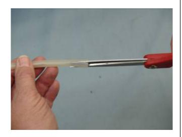
20. After splitting the silicon tubing cut off one side of the split section as shown. This will provide a relief section of the tubing for the nylon tie lock and insulate it from the metal pipe surface.
