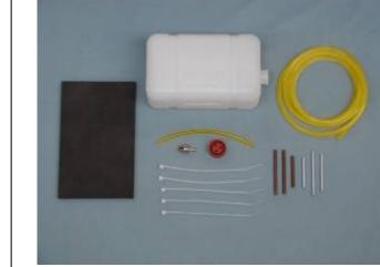
Assemble the fuel tank as shown below. Use large diameter tube for pick-up and small diameter tube for the vent. Secure the fuel tubing with nylon ties to the pick-up tube and clunk.
