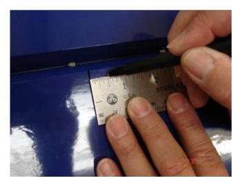
4. Tape leading edge of the elevator balance tab to the leading edge of the stab in the neutral position. Plug the servo into the receiver and turn on. Ensure the servo is centered and the servo arm is parallel to the elevator hinge line. Attach front ball link to servo arm. Adjust the length of the pushrod so that the leading edge of the control horns are aligned with the bottom leading edge of the elevator. Center the control horn over the mark and mark the
