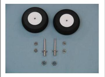
2. Use a drop of blue lock-tite on landing gear axle bolt before attaching the landing gear axle with the nylon lock nut.
