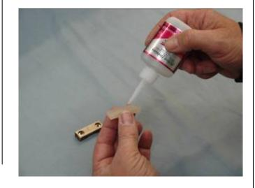
16. Glue the silicon rubber piece on top of the counter sunk holes on the plywood canister mounting bracket. This will seal the washers inside the canister bracket mount as shown.
