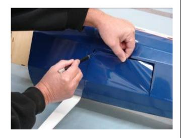
7. Use a hobby knife to remove the covering from the front former to the front of the land-ing gear cross brace as shown.
