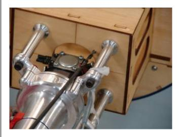
3. Attach the 2-56 ball link to the throttle pushrod and secure to the carburetor throttle arm with a 2-56 bolt and nylon lock nut.
