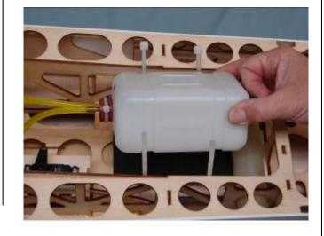
4. Install the fuel tubing as shown with small nylon ties. You will need an after market fuel T and fuel filling dot. Note: We recommend looping the vent line to the rear of the fuel tank as shown to prevent fuel spilling when the model tail is lifted or flying a down line.
