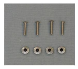
6. Slide the stab tube in the fuse stab tube sleeve. Slide the stabs on the stab tube and plug in the elevator servo plugs. Slide the rubber backed washers on the stab mounting bolts and insert bolts through the stab mounting tabs and into the fuse blind nuts. Tighten snugly but do not over tighten and crack the stab mounting tabs or the fuse sides.
