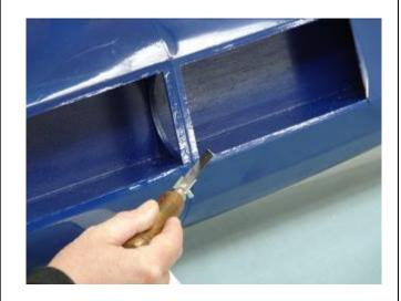
11. Cross braces removed from canister tunnel.
