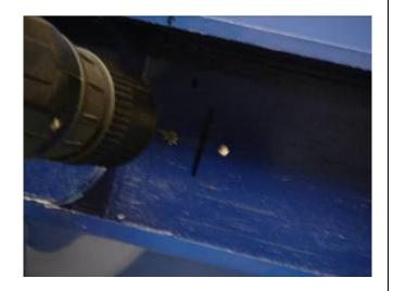
6. Locate the two plywood canister mounting doublers with pre-installed blind nuts as shown.
