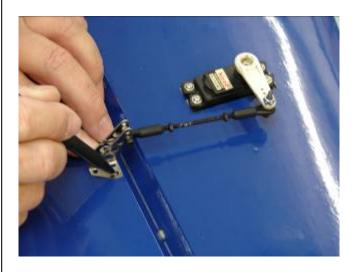
5. Use a 1/16" bit to drill the control horn mounting holes.
