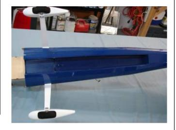
7. Iron the bottom covering to securely seal the covering to the bottom of the rear tuned pipe tunnel former.
