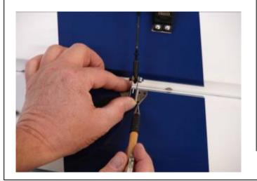
5. Use a 1/16" bit to drill the control horn mounting holes.
