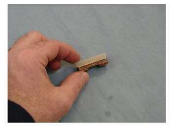
17. After the CA glue has fully cured, use a hobby knife to cut two small round holes in the silicon rubber. The holes should be just large enough to allow the heads of the canister mounting bolts to pass through the silicon rubber and seat against the washers inside.
