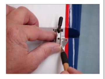
4. Use a 1/16 bit to drill control horn mounting holes.
