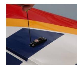
9. Aileron servo mounted in bottom of wing.
