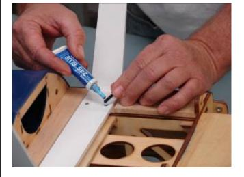
6. Bolt landing gear strut to fuse with 4 bolts and washers. Ensure tapered edge of the gear strut is facing toward the rear.
