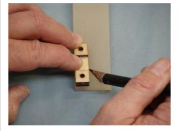
10. Use a hobby knife to cut the flat silicon rubber to match the size of the pipe mounting bracket.
