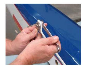
8. Install the inner wheel collar next to the axle bolt. Tighten the inner wheel collar in place. Install the wheel and outer wheel collar. Use blue lock-tite on the wheel collar set screw before final tightening.
