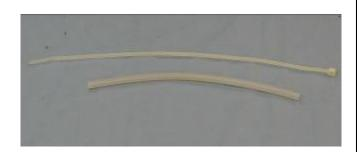
20. Use a pair of scissors to split one end of the silicon tubing in half approximately 3/4" deep as shown.
