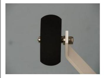
10. Slide the lock washer then the flat washer on the wheel pant mounting bolts. Use blue lock-tite on the bolts before final tightening.
