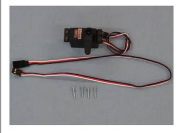
2. Layout the servo and extension on the wing to test fit the installation and ensure servo extension is the correct length.
