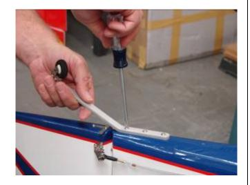
11. Attach the steering springs on both sides of the tail wheel to the rudder tiller and tail wheel tiller. Center the springs between both tillers.
