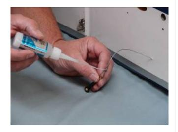
16. Hold the threaded coupler below the cable attach holes to thread into the ball link as shown. Do not hold coupler at the top where the cable hole is located. This may cause burrs on the coupler that can eventually cut the rudder pull cable.
