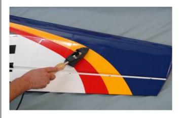
3. If bubbles persist, use a small pin to punch holes in the bubble to relieve trapped air and reheat.
