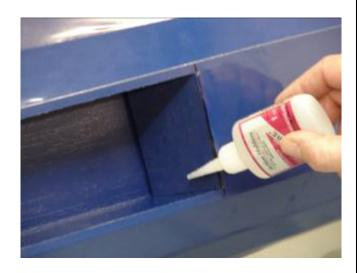
19. Rear canister tunnel former glued in place.
