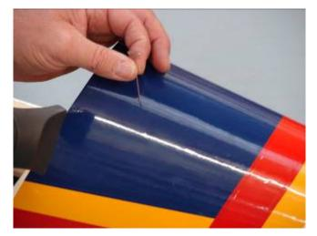
4. Use your heat gun with extreme caution. Take care not to apply too much heat to one area for long periods of time. This may cause the trim colors to over shrink and pull away leaving unsightly gaps on the color lines. The trim stripes are especially vulnerable to over shrinking.
