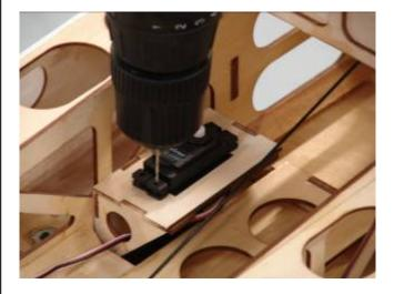
10. Install the servo using servo screws.
