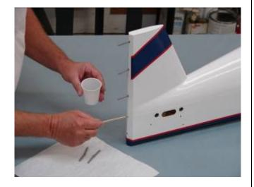
4. Epoxy the hinges into the fin first and allow epoxy to fully cure.
