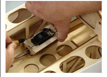
6. Prepare to epoxy the servo mounting tray to the fuse side. Apply epoxy to the back of the servo mounting tray.
