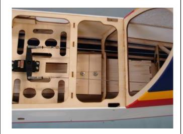
24. Install the pip mounting bolts from the inside the pipe tunnel and screw into the blind nuts to hold the doublers in place. Do not tighten. Tack glue the edges of the doublers to the top of the pipe tunnel with CA glue. Remove the bolts and glue the doublers securely in place. Do not allow CA glue to get into the blind nut threads.
