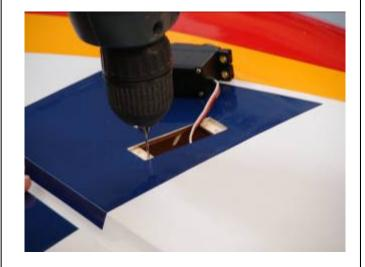
8. Install servo with servo mounting screws.
