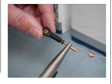
17. Attach ball link to rudder control horn on both sides of the rudder.
