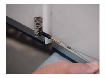
12. Loop the cable back through the brass swage tube as shown.
