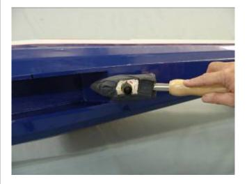
8. Dry fit the header and tuned pipe inside the tunnel and ensure there is clearance on all sides.
