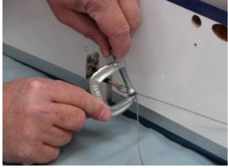
11. Attach a metal threaded RC link to each threaded coupler. Attach the RC links to the rudder servo arm and then attach the servo arm to the rudder servo as shown. A 2 3/4" to 3" arm is recommended.
