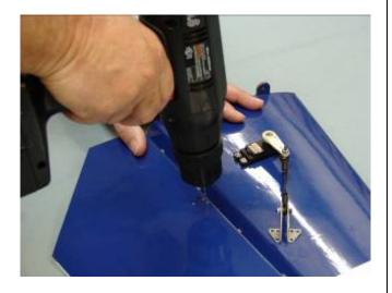
6. Mount the control horn using six wood screws as shown. A 1 1/2" servo arm is recommended to achieve full deflection of the elevator bevel.
