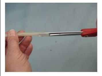
21. After splitting the silicon tubing cut off one side of the split section as shown. This will provide a relief section of the tubing for the nylon tie lock and insulate it from the metal canister surface.
