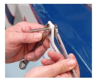
4. Snug axle to gear strut with the flat sides vertical. Align axle with wheel pant slot.
