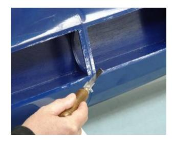
6. Covering and cross braces removed from tuned pipe tunnel.
