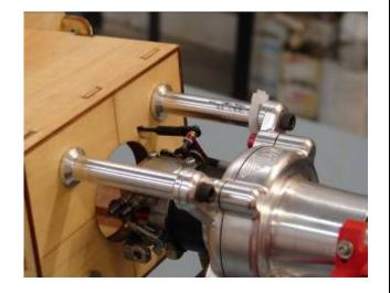
4. The throttle servo is mounted on the side of the fuse that aligns with the engine carburetor throttle arm. Insert the throttle servo into the appropriate throttle servo mounting tray with the output arm forward. Insert the throttle pushrod into the servo arm easy link and dry fit inside the fuse. Align the servo tray so there is no binding on the throttle pushrod.
