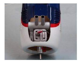
17. Final cowl installation with engine muffler.
