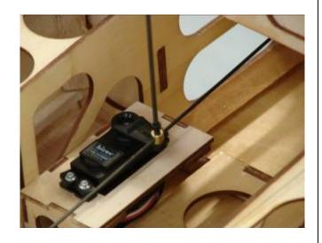
12. Cut off the excess pushrod wire as shown.
