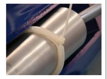
28. Cut off excess nylon tie as shown.
