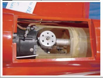
Epoxy the muffler support to the rear liner. Refer to drawing#1 for detail.
