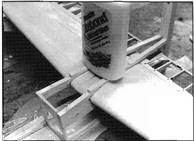
Joined stab and elevator are glued in place early in fuselage construction.
