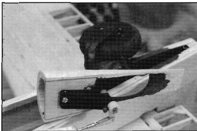
Balsa tail wheel pushrod is attached to cut-down nose wheel steering arm.
