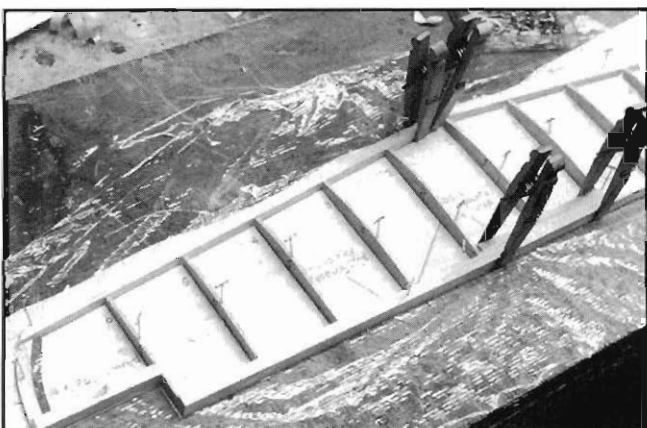
Stabilizer is built in two clamshell halves.
