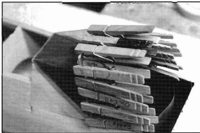
Painted frame is glued to windscreen. A lot of clothespins hold while glue sets.
