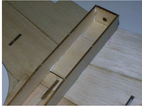
Figure 4.4: Reinforcement sheets glued
