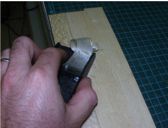
Figure 2.6: Shaping the elevator
