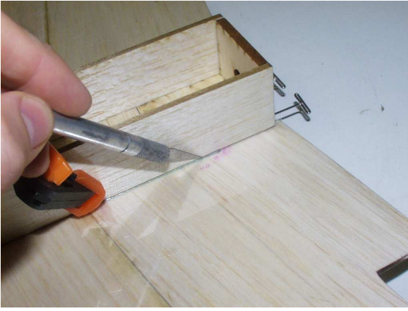
Figure 4.3: Score and remove excess covering
