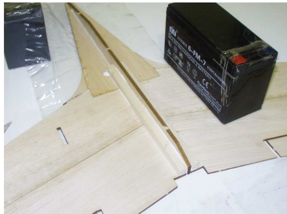
Figure 3.14: Reinforcement stock added
