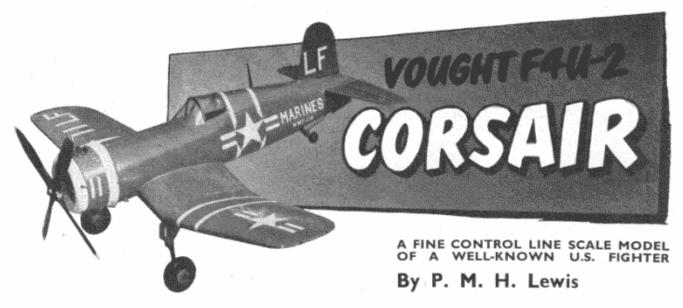
THE Vought F4U-4 Corsair, fitted with the 2,000 h.p. Pratt and Whitney Double Wasp R2800 motor, was one of the most successful naval fighters in use with the Allies during the 1939-45 war. With a span of 40 ft. and carrying six .5 cal. machine guns the top speed was approximately 390 m.p.h. The model described here is of a machine in use in 1951 with a U.S. Marine Corps Fighter Unit (V.M.F.) and is designed around the 1.5 c.c. Allbon Javelin.
