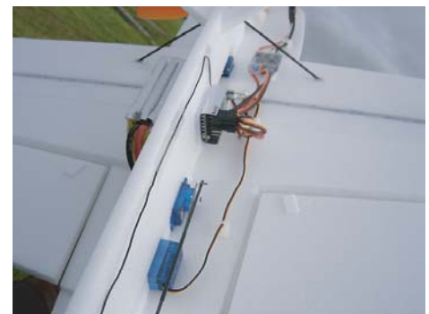
Not speed control and Rx locations. Battery is on the opposite side.
