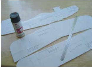
Lighty coat back of plan parts with Spray Adhesive, apply each part to Depron. Carefully cut each part out using a strightedge and #11 Xacto.
