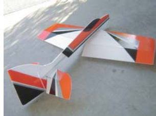
Colored Zagi tape works great for trim. It's best to trim each part before assembly.
