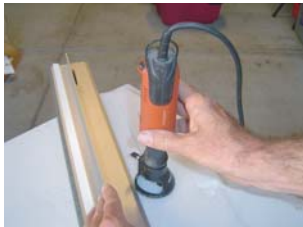
A Rotary Tool Cutting Adapter is perfect for clean easy to make grooves for Fiber Carbon rod stiffeners.
