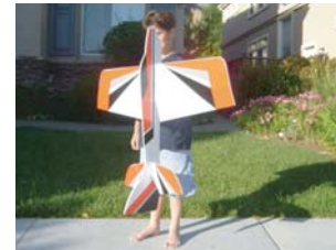
Colored Zagi tape works great for trim. It's best to trim each part before assembly.
