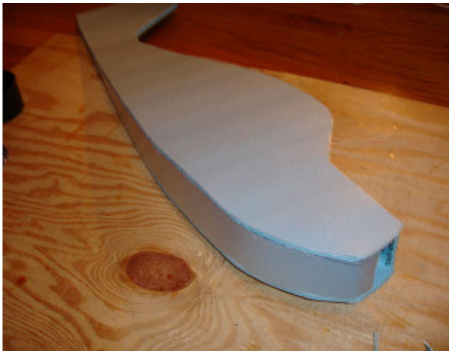
Bottom fuse completed.
