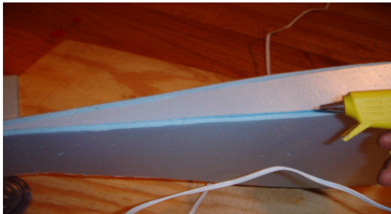
Position the bottom fuselage and hot glue.
