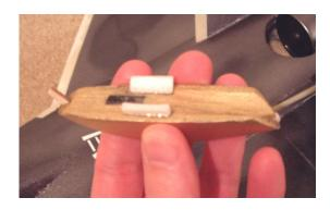
Add tabs from scrap material to attach the canopy to the forward fuselage.
