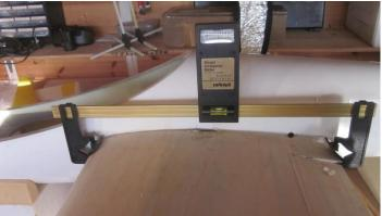
Stefano has confirmed the incidences: Wing about 0.8°, tailplane zero. The front incidence pin hole is OK, then, and the rear one can be drilled correctly in the fairing facing.
