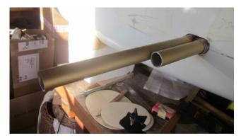
Looks OK inside, too. I had hoped that I'd be able to bond the joiner tubes to the crutch, and here you see it. Spot on! (Nothing is glued in place yet.) Note the coat of primer on the crutch.
