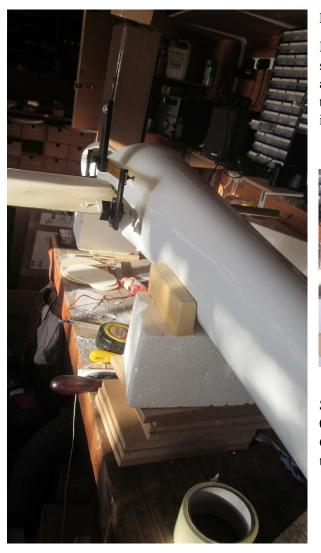
Must get in touch with Stefano to check what the suggested wing and tail incidences are! At this point I also noticed that there is a gap of about an inch at the trailing edge of the wing, so that the hole for the rear incidence pin will be covered by the fairing!
