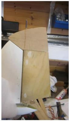
Having atoned for past errors, it's time to get on with the build. Some holes are needed to accommodate wing joiners and incidence pins. I've drilled the joiner holes a little oversize so that adjustments can readily be made.
