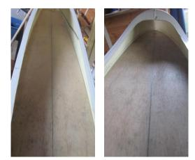
The crutch is (intentionally) a tiny bit undersize (glue's got to go somewhere!), so that the line is above it. Fortunately, it is reasonably uniform from nose to tail. The other good thing is that it is possible to get it in and out again. Correct placement will be ensured by the fittings for the aerotow in the nose, and for the bungee release amidships.
