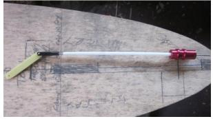
Graupner aerotow, with plastic tube guide, and a G10 actuator arm to convert the rotary motion of the servo arm to linear.
