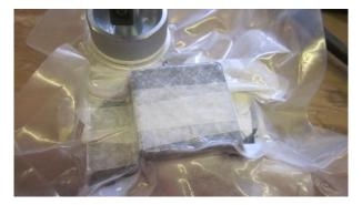
Three layers of carbon cloth and loads of epoxy in a vacuum bag.
