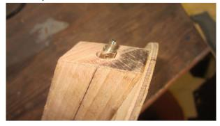
Here's the business end, with bungee pin in place. I'll probably grind off the thread from the pin. It is a 70mm piece of chrome plated steel that I found in a box labelled "Interesting metal".
