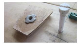
The blind nut is fitted to the ply plate with epoxy and microballoons. Plate is shaped to be a good fit in the rear of the fuselage.
