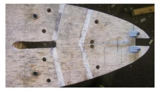
I had to rout out a couple of channels to accommodate the ties that hold the batteries to the plate.
