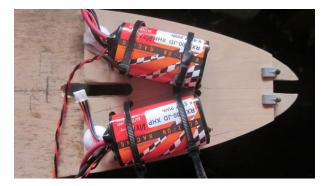
Here's the removable plate that fits in the nose, and carries batteries and nose weight. It's secured with two nylon bolts into blind nuts in the crutch, and those two plastic cable ties, that I modified to take the plate. They are screwed and glued to the crutch, and the plate slips under them. Note the holes for the tow release (right) and its actuation system (left).
