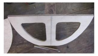
Some lightening holes (also good for access and wire runs), adjustment of angles and glue and the release is done. The top will need narrowing to get the level of the crutch right.
