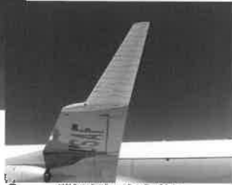
NASA Dryden Flight Research Center Photo Collection http://www.dfrc.nasa.gov/gallery/photo/index.html NASA Photo: 027811481 Date: 1978 X-45 in flight - closeup of winglet with attached tabs
