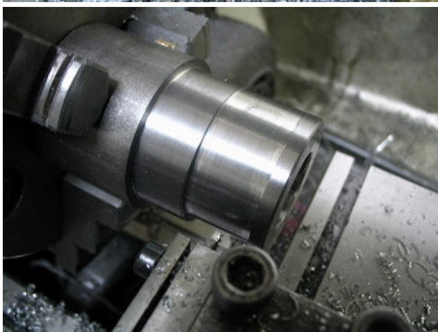
9. (ECCENTRIC CAM) Turning of the eccentric cam. The material is free cutting steel of the 40mm diameter.
