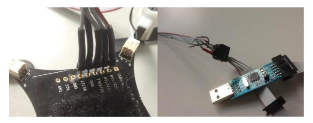
The 6-pin connector oft he USasp hast he following pin assignment. The Pins you need to connect also marked on the PocketQuad Board. Warning VCC is not required!
