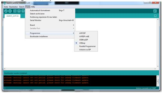
5. Choose under the Tools tab "install Bootlader", this starts the upload. This may takes several minutes. After the upload you can use the integrated USB-Port to upload new Code to your PocketQuad. (New code to bind the receiver, for example).
