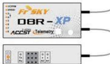
The FrSky telemetry receiver then sends the data via the radio link to your FrSky 2.4Ghz telemetry Tx's such as the DHT-U module, LCD display connected to a DHT or telemetry modified receiver with DHT and ER9X.
