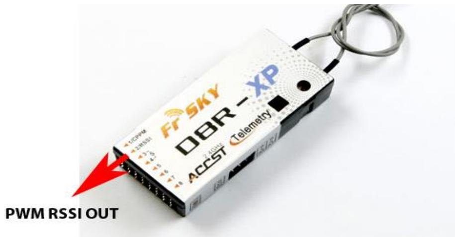
To work with MinimOSD and a PWM RSSI input, an alternative version of the MinimOSD is available here <http://code.google.com/p/minimosd-extra/>. You will need to configure and install as detailed in the link. (If you do not require RSSI then the standard OS Build for the MinimOSD will be fine). To configure the OSD you will need an FTDI adapter to load and configure the firmware.
