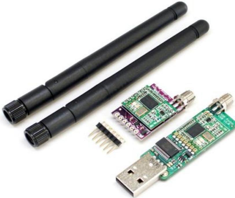
The 3DR Radios connect to the telemetry port on the APM 2.5, some of the clone radios now appearing on the market have different connections from shown above, the units currently supplied by Rctimer in their latest bundles have a socket similar to the GPS. The cable supplied by Rctimer as part of their bundle offer makes the radios wiring plug and play. If you source your radios elsewhere or use genuine radios then you will need to make a suitable cable.
