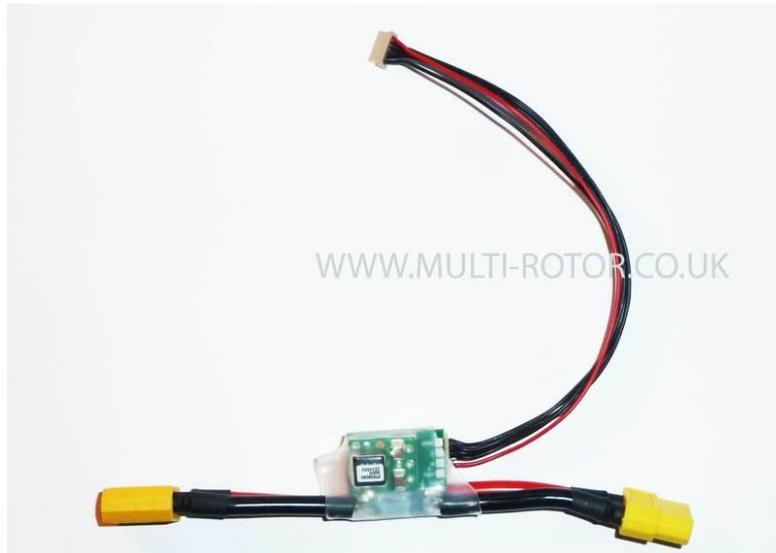
The new module plugs into what was previously known as the mystery port or power port. It is available with XT60 or deans connectors. It is a simple way of providing the APM 2.5 with clean power from a LiPo battery as well as monitoring current consumption and battery voltage measurements.
