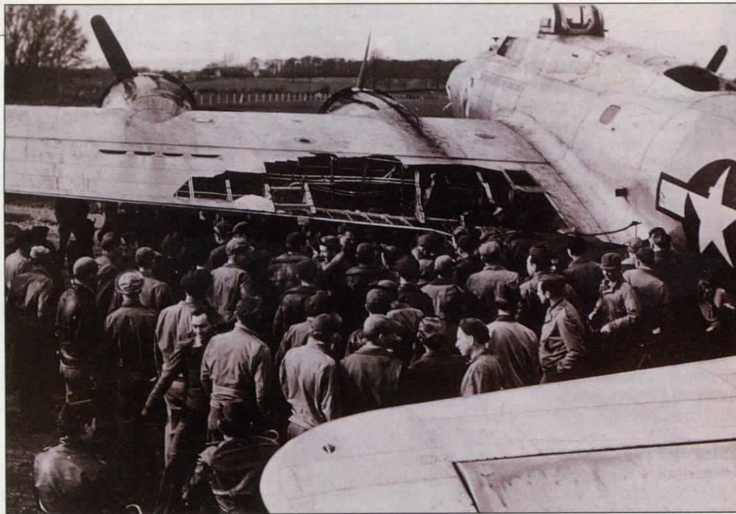
ABOVE A B-17 returns from a mission with heavy damage to the port wing, probably inflicted by a single hit from the Me 262's 30mm cannon.
