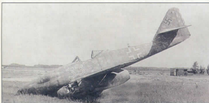
BELOW An Me 262A-1a/U3 of the tactical reconnaissance unit Kommando Braunnegg. Note the large bulge on the top side of the nose, covering the film magazine of the port camera.
