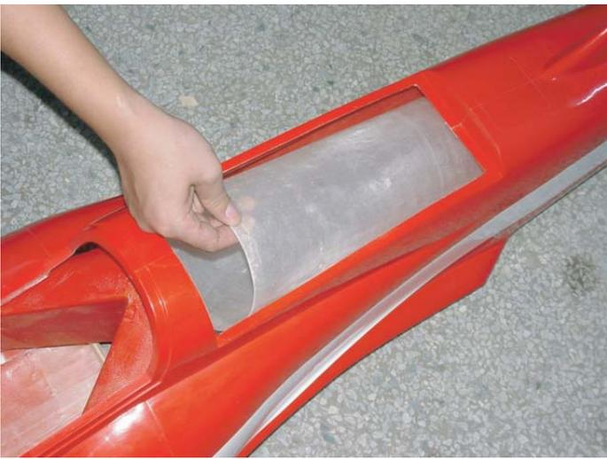
**29** Mark the exceed portion on the front liner and cut it out.
