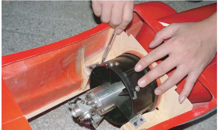
Photo shown is the OS .46 VX-DF engine and Turbax 48 fan. Turbax 48 fan and K&B .48 ducted fan engine may be used as alternatives.
