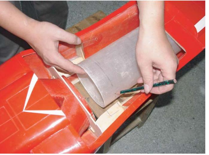
**30** Cut out the hole on the front liner for engine cap. Refer to Fig #1 for detail.
