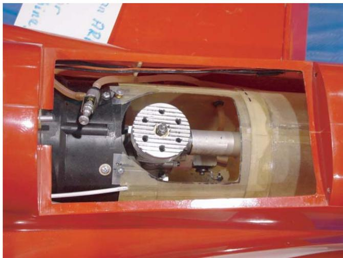
**39** Epoxy the muffler support to the rear liner. Refer to drawing#1 for detail.
