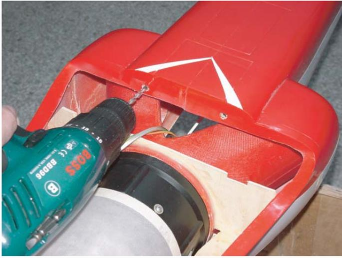
**14** Drill the hole on leading edge and epoxy two pieces wooden dowels in place.
