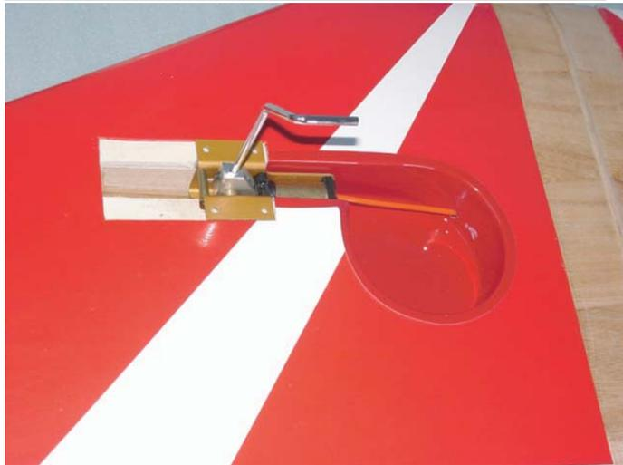
**12** Remove the covering film and glue the plywood doubler.
