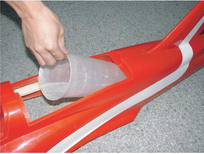
**27** The exhaust liner should come out from the fuselage for 1/4".
