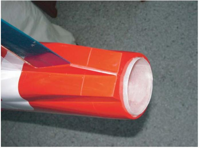
**28** Insert the front exhaust liner. It should fit on the bell mouth of the rear liner.
