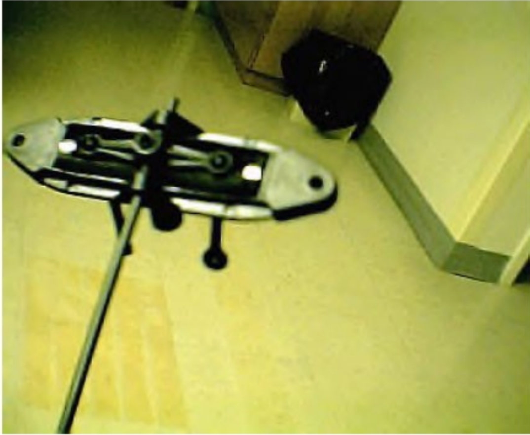
You can see the 2 bearings here, center flybar and put paddles back on...
