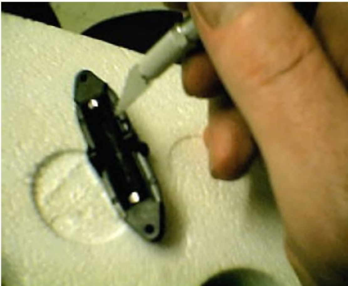
The flybar/stabilizer yoke must not bind like this.
