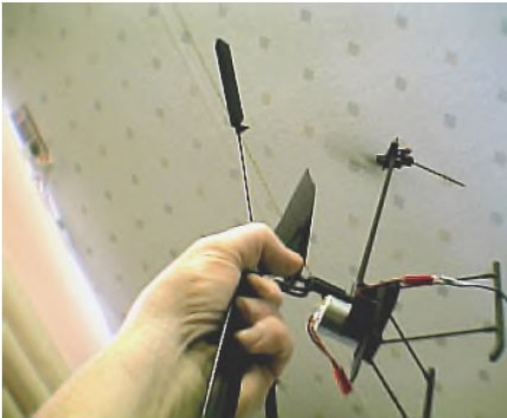
plugged into tail motor, run it up and see how it works. Should be smooth if balanced. If not, check again. Check gear mesh
